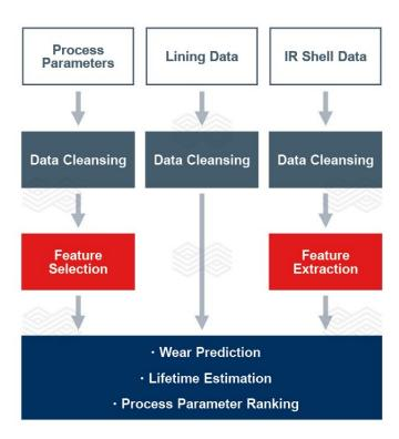
These measurements represent the minimal lining thickness for each of the 20 brick layers and 8 segments per layer of the lower part of the vessel sidewall. Additionally, the bottom lining thickness was also measured. Several prediction models were created for areas with large wear rates, which are called hot spots (HS).
