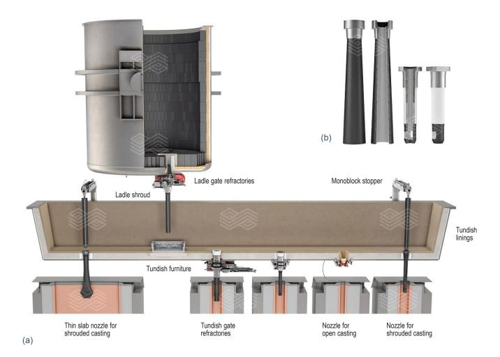
For better thermal shock resistance the carbon content of flow control products is rather high, at 20-30 wt.%, which also results in a high thermal conductivity of these products. Consequently, some measures have been used to minimize the heat losses through the refractory walls. RHI Magnesita has developed special liner materials that are applied inside the product bore with improved insulating properties for LS and SEN to achieve this goal.
