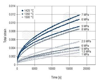
Total strain curves for a defined temperature versus testing time derived experimentally and through FEA simulation are shown in Figure 6, Figure 8, and Figure 9. As depicted in Figure 6, the material showed distinctive creep behaviour at 1350 °C. The creep parameters which were found for 1350 °C cover the whole load range of 5, 6, and 8 MPa, resulting in a good agreement of the experimental and the simulated 8 MPa curve.
