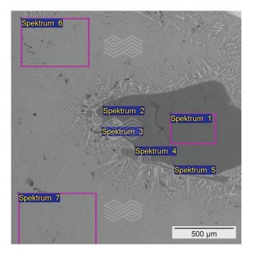
Based on the matrix analysis, the average MgO concentration in the bulk slag did not exceed 4 wt.% (Table VIII), which is lower than the desired MgO content of 7 wt.% (Table IX). Microscopically, it could be clearly seen that the fused magnesia had not dissolved completely within the holding time, although it was 10 minutes longer than in the test with caustic magnesia.
