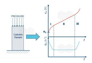
tertiary creep stage, which would cause the collapse of the structure. In some unique cases, for example in a regenerator superstructure, the weight load of the checker bricks in combination with elevated temperatures could cause stresses relevant for creep that will not disappear with increasing deformation. Hence, special care has to be taken when selecting materials for such structures in order to avoid creep-induced failure.
