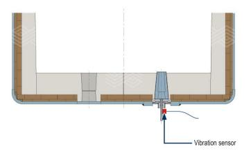
For this method, a vibration sensor is mounted to the connecting pipe of a purging plug, detecting mechanical waves running from the plug surface through the plug to the sensor. These mechanical waves are generated by the impact of the melt on the plug surface after the gas bubbles have detached from the plug surface and the melt falls back. For the vibration signal the normalized amplitude over the time is recorded in a vibration spectra, an example is given in Figure 2.
