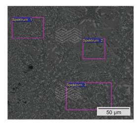
**Table VI.**EDX analysis results of the synthetic slag heated with caustic magnesia, showing the average results of obtained spectra. Holding time 10 minutes.
