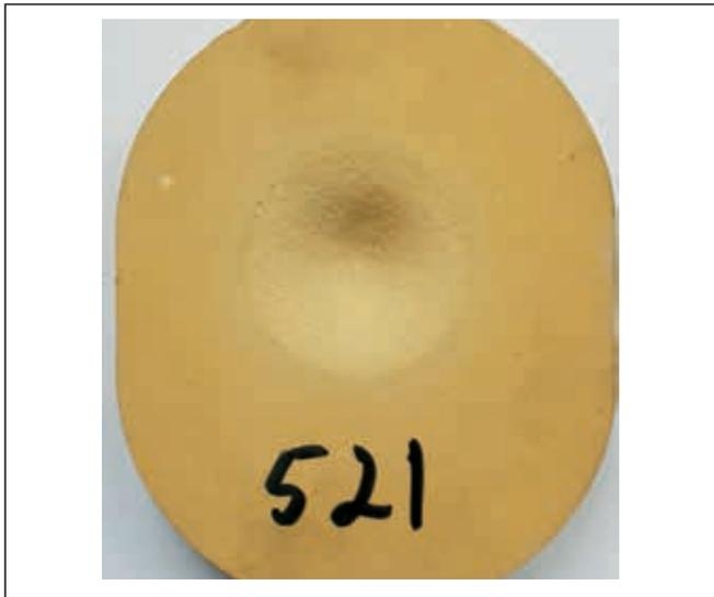
Figure 11. Sample after high temperature abrasion test.
