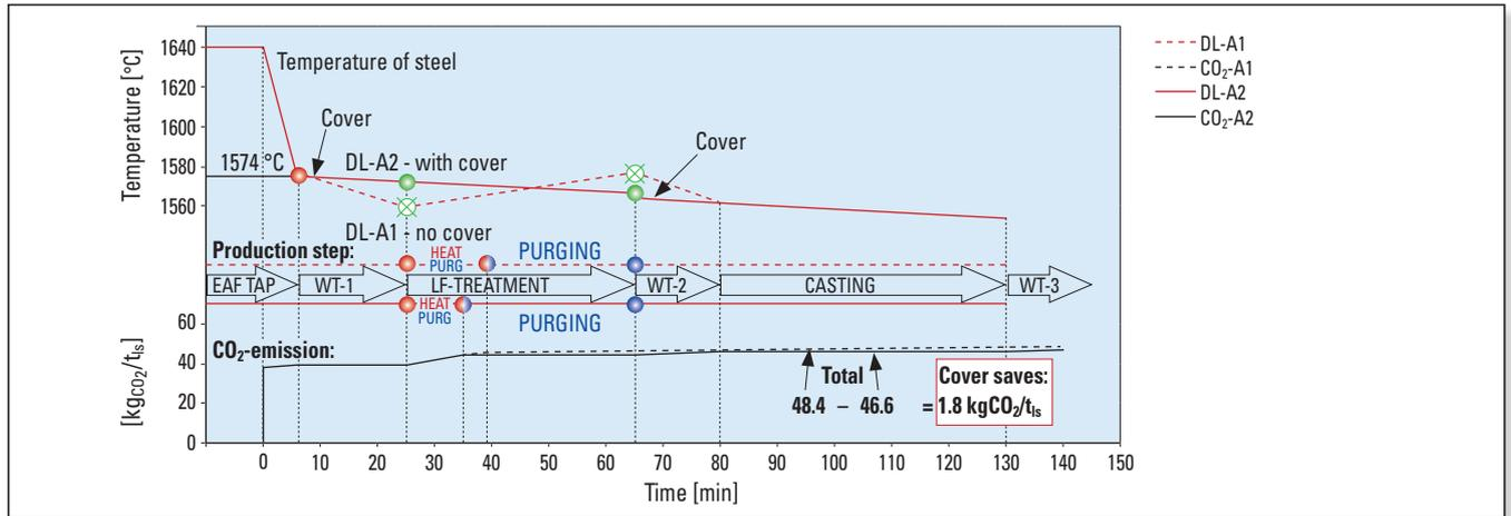
Figure 6. Time-temperature charts and CO<sub>2</sub> emissions during one heat for cases DL-A1 (doloma-lime, no cover) and DL-A2 (doloma lime, with cover) due to the corresponding production step [6].
