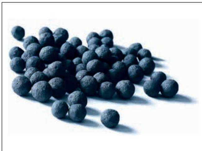
**Figure 1.** Picture of iron ore pellets after treatment. (Courtesy of Outotec GmbH & Co. KG).
