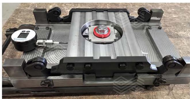
As shown in Figure 7, the tension forces measured during the functional model tests were very well within the test predictions. Even for failure cases such as loss of a lever or a spring, the tests showed that the tension system still provides a sufficiently uniform pressure to the plates.
