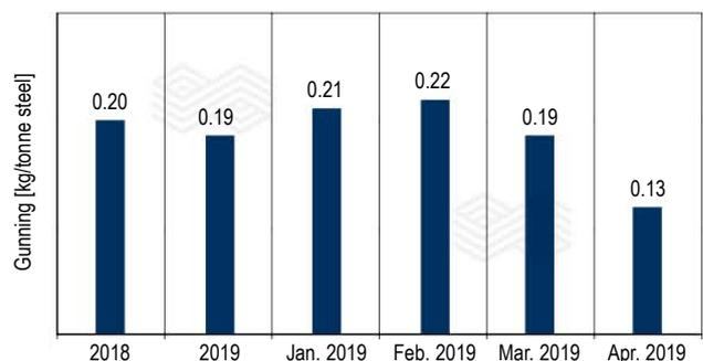
The long-term average consumption had been 0.21 kg/tonne steel; however, during the trial period only 0.13 kg/tonne steel was used. Overall, this meant a 38% reduction of refractory material use as well as a significantly lower number of gunning applications, thus reducing both time loss in production and manpower spent on maintenance.
