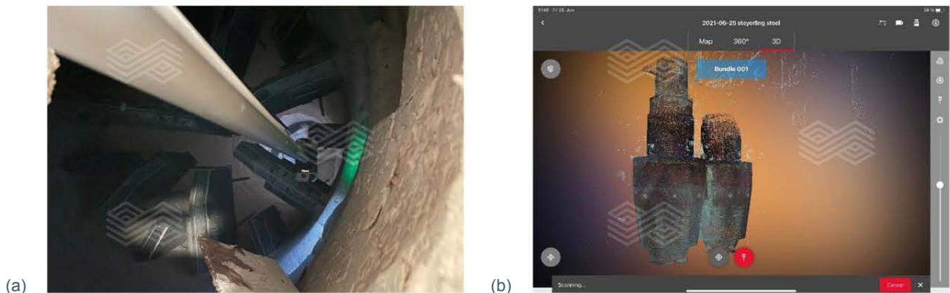
While LES is optimal for vessel inspection under cold conditions, the new QCK (Quick Check) technology is used for hot vessel measurements. This technology is based on stereoscopic cameras and is a very interesting alternative to laser scans in hot conditions, being much faster and more accurate (Figure 5).
