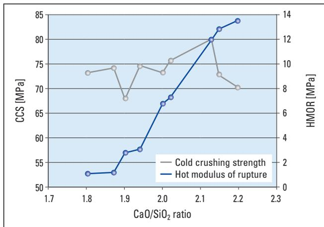
**Figure 2.** Variation in cold crushing strength (CCS) and hot modulus of rupture (HMOR) of magnesia bricks containing an increasing C/S ratio.
