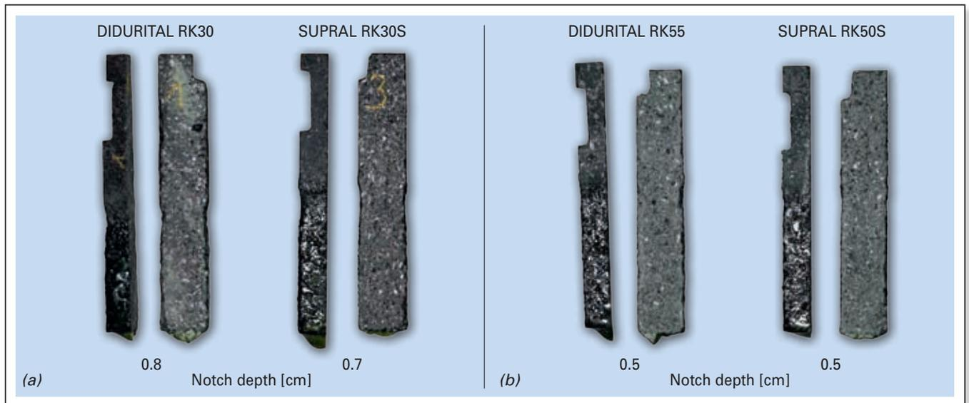
**Figure 10.** Corrosion behaviour of (a) DIDURITAL RK30 and (b) DIDURITAL RK55 in C-glass. In the static plate corrosion tests DIDURITAL RK30 and DIDURITAL RK55 were compared to the analogous pressed SUPRAL RK30S and SUPRAL RK50S grades, respectively, for 96 hours at 1500 °C.
