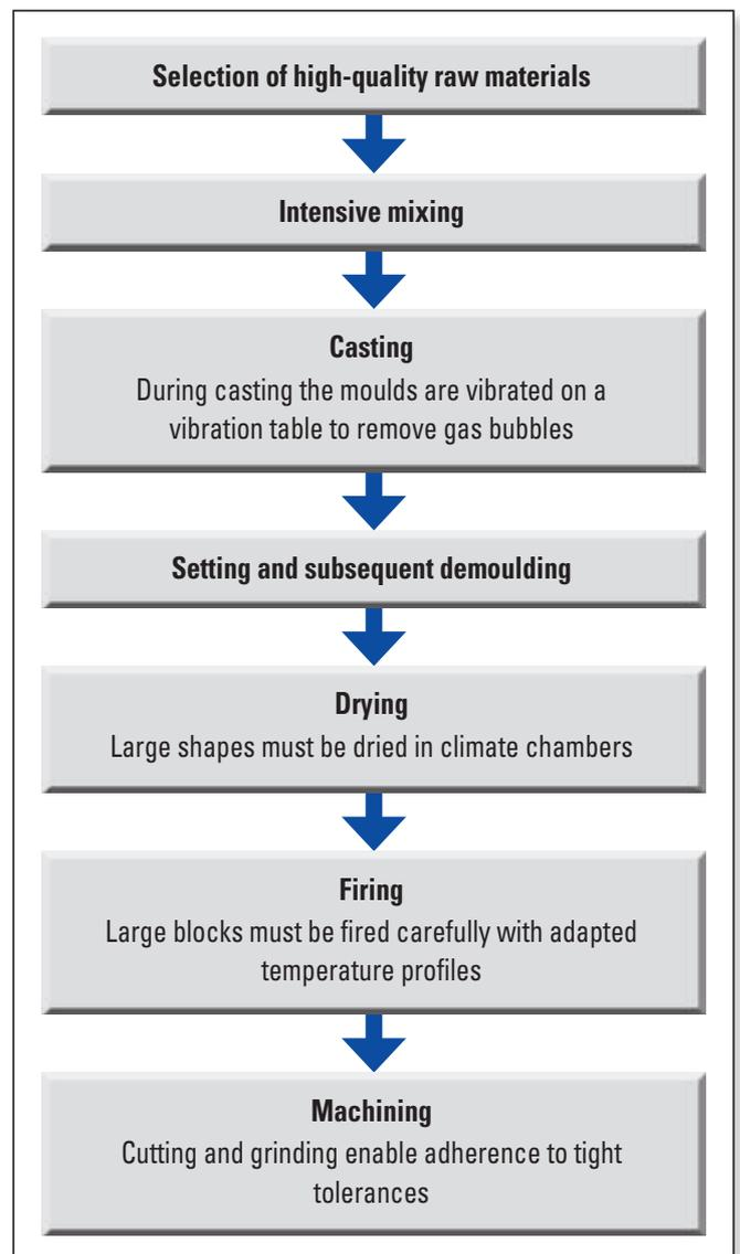
Figure 1. Vibrocasting production process.
