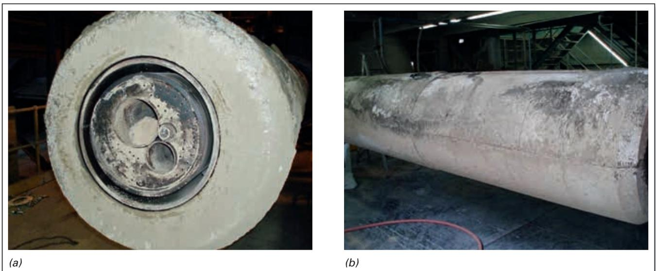
**Figure 5.** Burner tip lined with CARSIT SOL M10-5 V in perfect condition after 7 months in operation. Traditional low-cement castables resulted in a lifetime of only 4 months.
