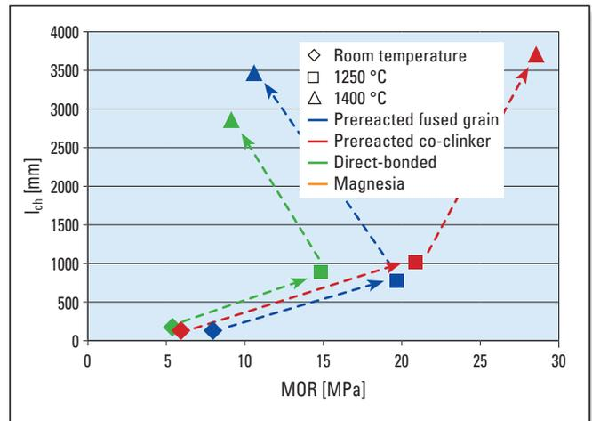
**Figure 9.** Comparison of the relationship between the characteristic length,  $l_{ch}$ , and MOR for the MCr 50 types examined at room temperature, 1250 °C, and 1400 °C.
