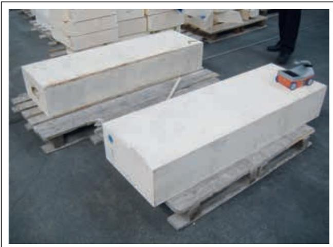
**Figure 2.** Tested fused cast blocks: The FVB with the radar measuring instrument (foreground) and the CRB.
