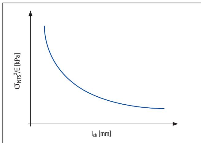
Figure 4. Inverse trend between  $\sigma_{NTS}^2/E$  and the characteristic length,  $l_{ch}$ . A lower  $l_{ch}$  indicates a more brittle behaviour.
