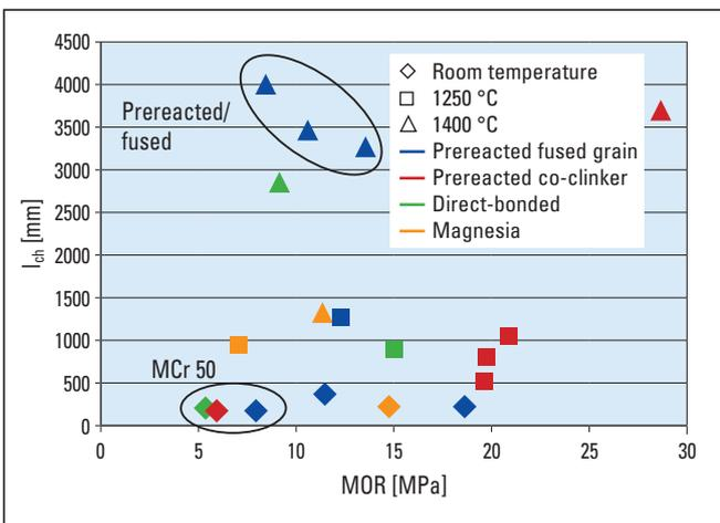
**Figure 8.** Relationship between the characteristic length,  $l_{ch}$ , and MOR for all the brick types examined at room temperature, 1250 °C, and 1400 °C.
