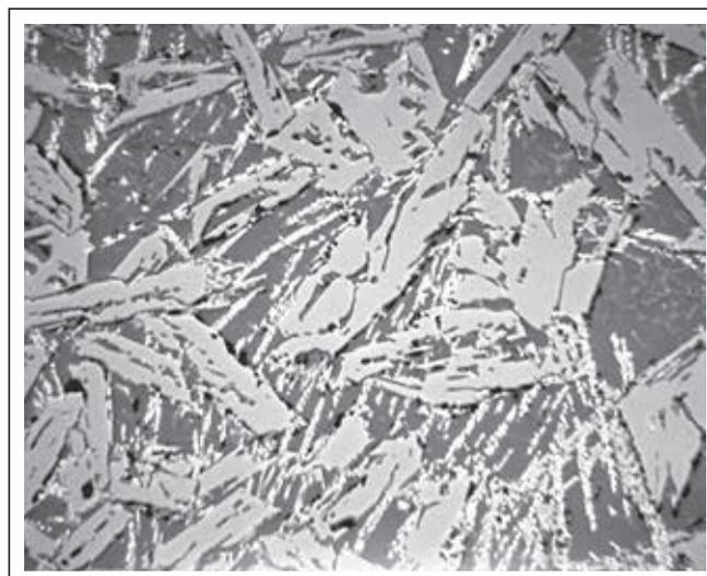
**Figure 3.** Microstructure of REFEL 1616ULX. Corundum crystals (light grey), zirconia dendrites (white), and a sodium aluminosilicate glassy phase (dark grey) are clearly visible.
