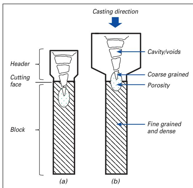
**Figure 1.** Correlation between the cavity volume and casting header size. (a) the block contains a reduced size cavity and (b) the block is cavity-free because the larger header compensates the volume shrinkage.
