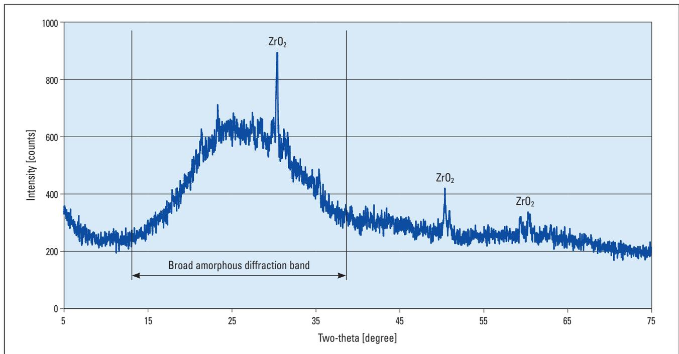
Figure 5. XRD scan of the white defect solid inclusions.
