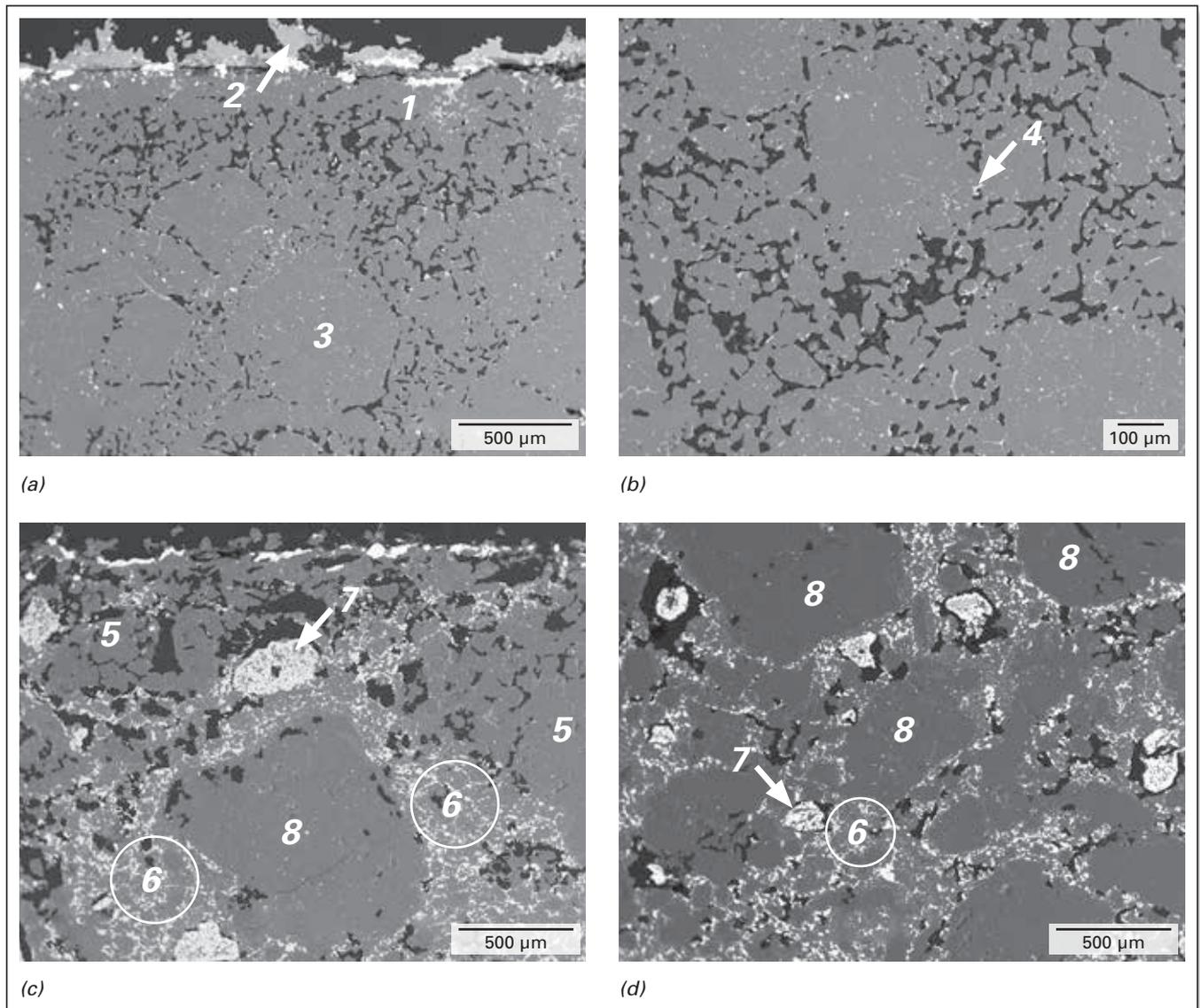
**Figure 10.** Scanning electron micrographs of used ANKER DG1 and RUBINAL EZ (a,c) at the hot face and (b,d) 20 mm from the hot face, respectively. Densification (1), surface deposits (2), strong bonding between the magnesia grains (3), dicalcium silicate (4), corroded magnesia (5), forsterite bonding matrix (6), zirconia (7), and intact magnesia grains (8) are indicated.
