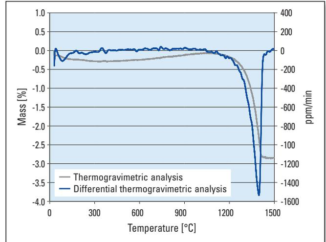
**Figure 11.** Thermogravimetric and differential thermogravimetric analyses of RUBINAL EZ.
