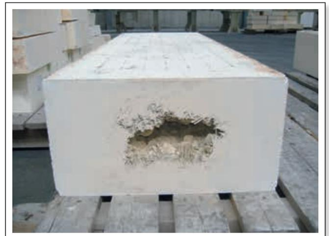
**Figure 5.** Cut face between the block and casting header of a CRB. The residual cavity is visible, which is typical for CRBs. Cross section  $250 \times 460 \text{ mm}^2$ .
