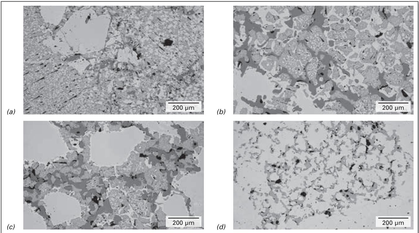
**Figure 1.** Microstructures of the different magnesia-chromite and magnesia brick types comprising (a) prereacted fused grain magnesia-chromite and chrome ore, (b) prereacted co-clinker magnesia-chromite (OXICROM) and chrome ore, (c) direct-bonded magnesia-chromite and chrome ore, and (d) pure magnesia.
