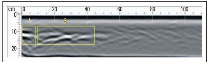
**Figure 7.** Radar image of the CRB. Visible black-white interferences indicate the location of (1) a void and (2) porosity.
