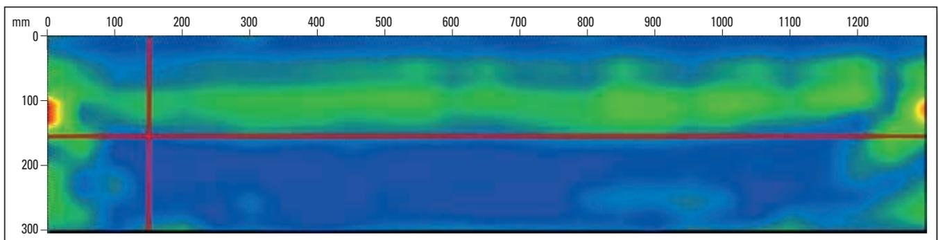
**Figure 9.** Ultrasound image of the FVB. The various colourations are signal interferences and are not related to block flaws.
