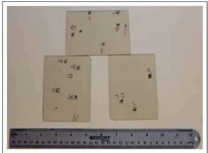
**Figure 13.** Cover glass samples with stone defects circled on the pieces.
