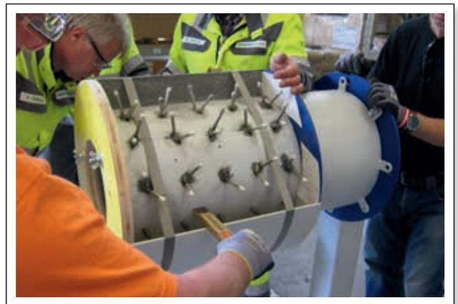
Figure 2. Preparation of a mould for castable installation.
