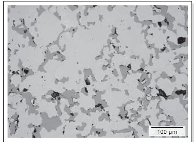
**Figure 3.** Direct bonding between MgO-MgO in ANKER DG1.
