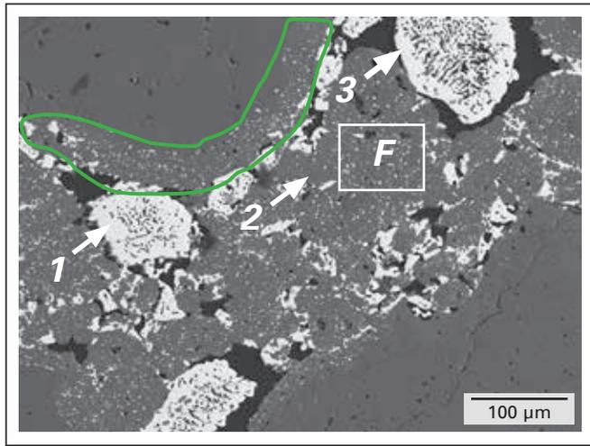
**Figure 5.** Scanning electron micrograph of unused RUBINAL EZ.  $ZrO_2$  (points 1 and 3), forsterite (point 2), and a mixture of forsterite and  $ZrO_2$  (area F) are indicated. A rim of forsterite containing tiny  $ZrO_2$  crystals was detected around the  $MgO$  grains (green line).
