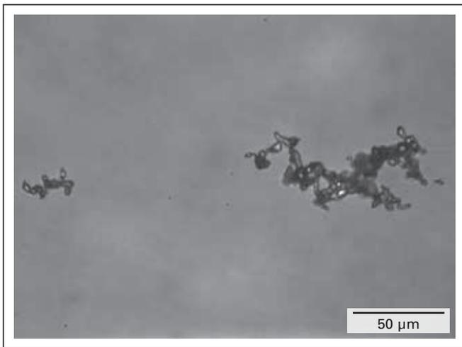
**Figure 14.** Stereoscopic micrograph of a stone with branching patterns within the glass wall thickness.
