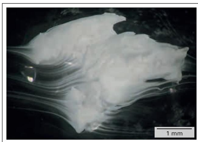
Figure 1. Stereoscopic micrograph of the white defect.
