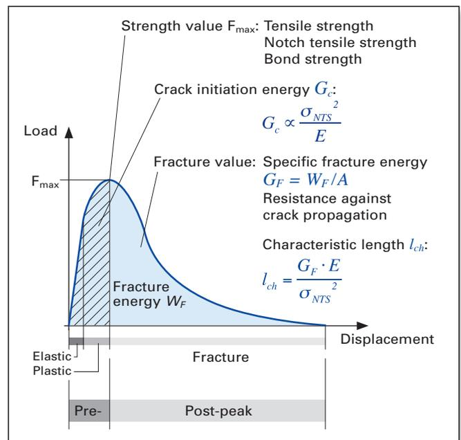
**Figure 3.** Typical load-displacement graph of a refractory material generated using the wedge splitting test according to Tschegg [5].
