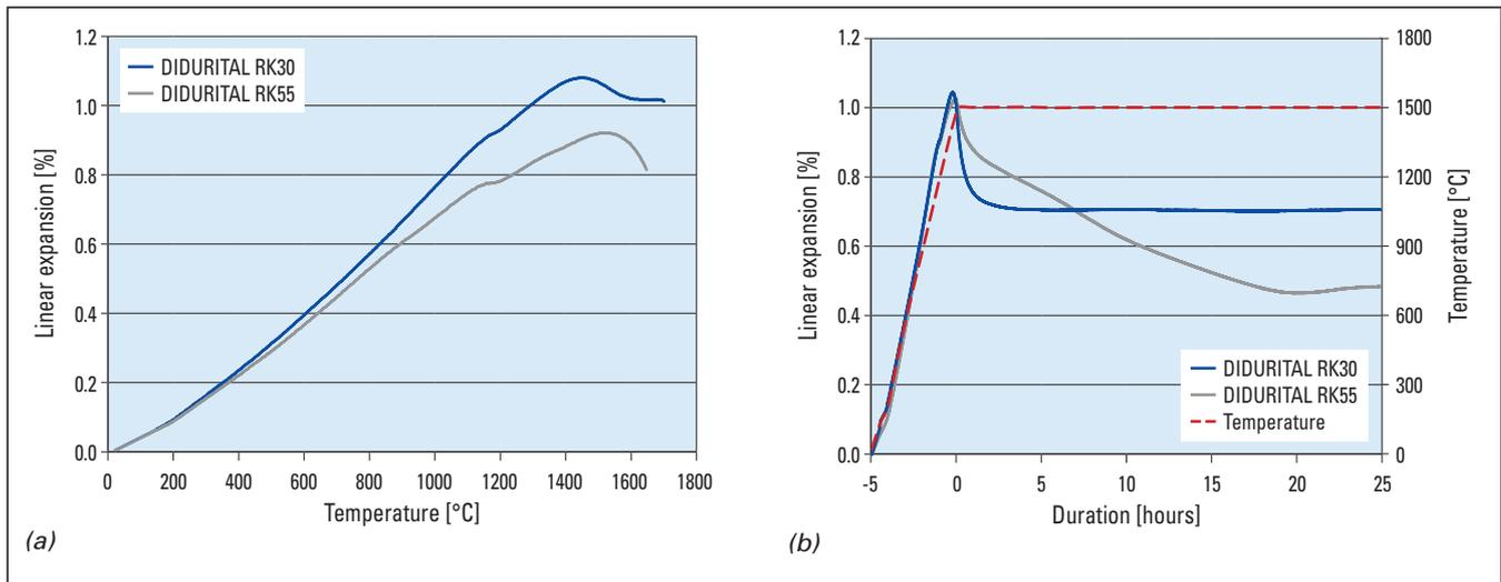
**Figure 11.** Typical (a) refractoriness under load values and (b) creep data for DIDURITAL RK30 and DIDURITAL RK55.
