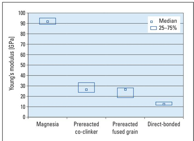
Figure 5. Box plot of the Young’s modulus results determined nondestructively using the ultrasonic and resonant frequency test methods at room temperature.
