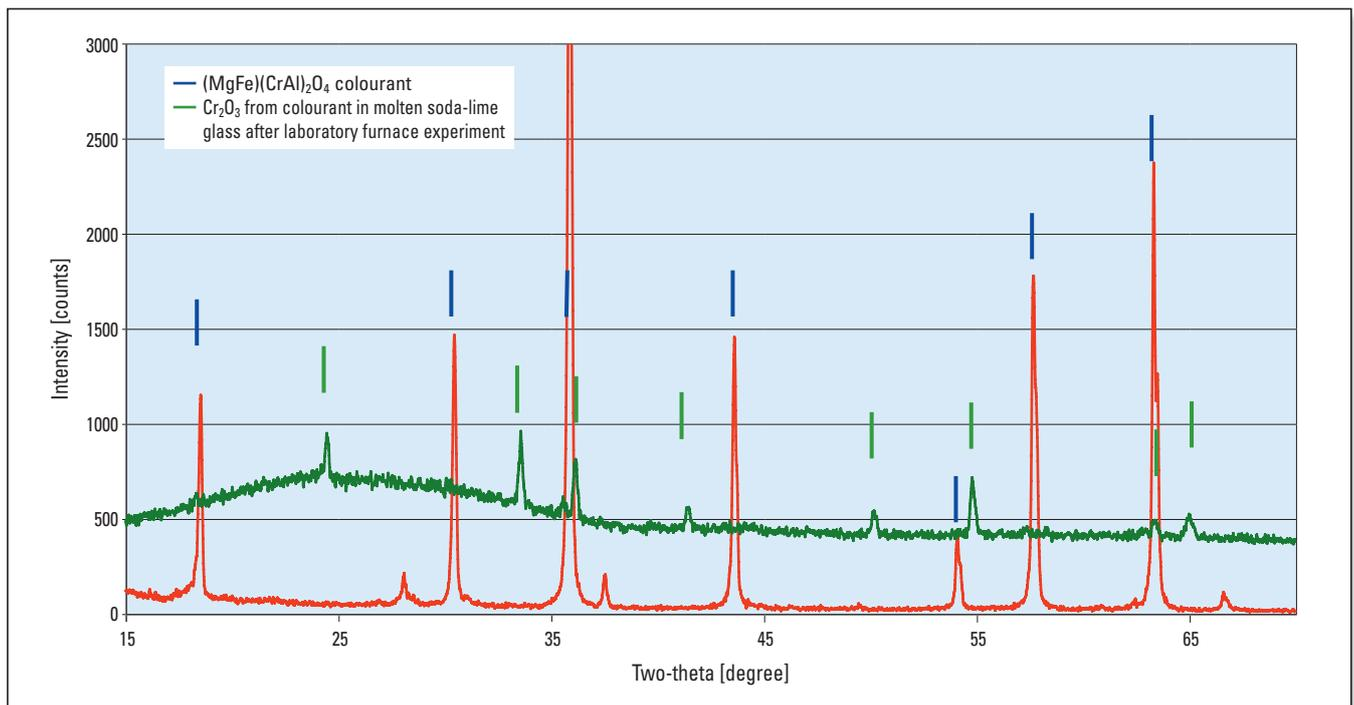
**Figure 11.** Superimposed XRD traces of the original colourant powder (red trace) and a sample of the molten soda-lime glass with the dissociated chrome iron spinel colourant (green trace) showing the peaks associated with crystalline phases. The chromite colourant completely dissociated to chromium oxide in the soda-lime glass cullet after 1.5 hours at 1490 °C.
