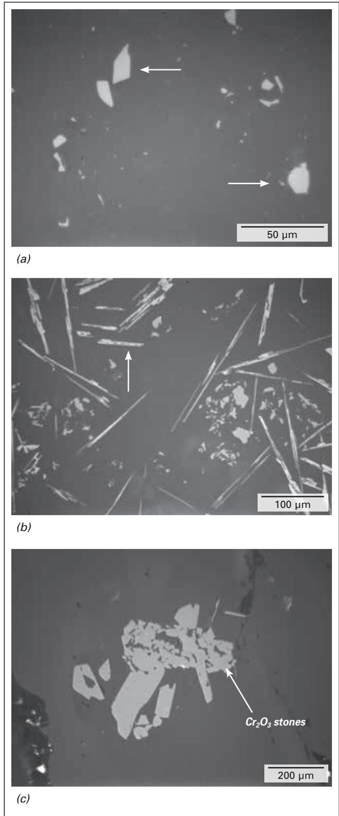
**Figure 10.** Reflected light micrographs of the (a) colourant (arrows), (b) results of the laboratory furnace test showing chromium oxide blades (arrow), and (c) a stone defect from the green bottle glass.
