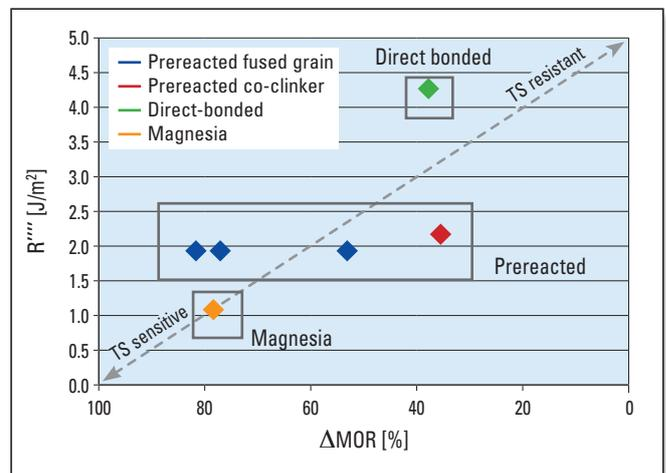
**Figure 10.** Relationship between the thermal shock resistance parameter  $R'''$  and the  $\Delta$ MOR, an indicator of thermal shock damage.
