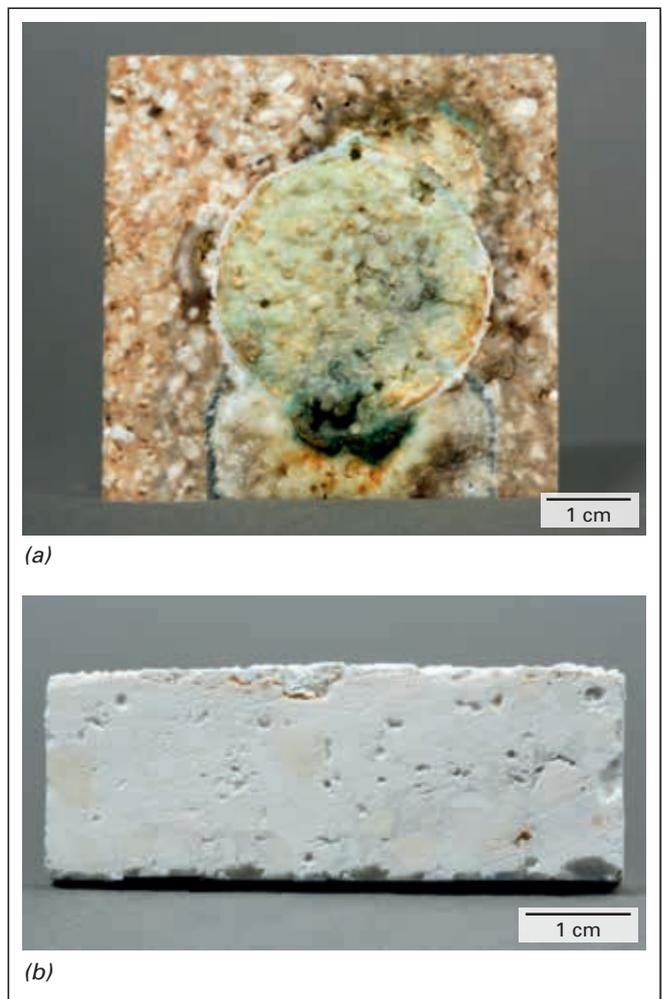
Figure 8. DIDURITAL S67 test sample after alkali attack. The test was performed in sodium carbonate vapour at 1370 °C for 72 hours. (a) surface and (b) cut sample.
