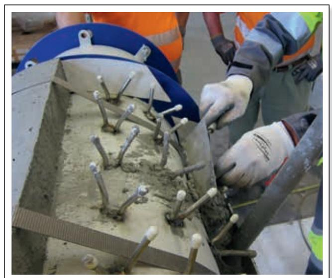
Figure 3. Casting and vibrating the sol-bonded CARSIT SOL M10-6 castable.
