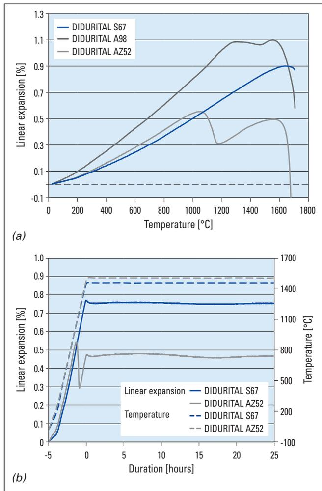
Figure 7. Typical (a) refractoriness under load values and (b) creep data for DIDURITAL AZ52, DIDURITAL S67, and DIDURITAL A98.
