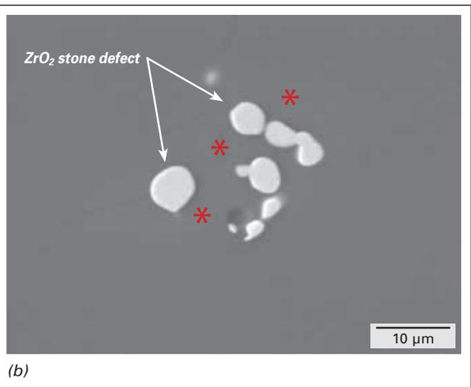
**Figure 15.** SEM backscatter micrographs of polished sections across the stone body. The red asterisks are glass regions within the stone. EDS analyses confirmed the stones to be zirconia.
