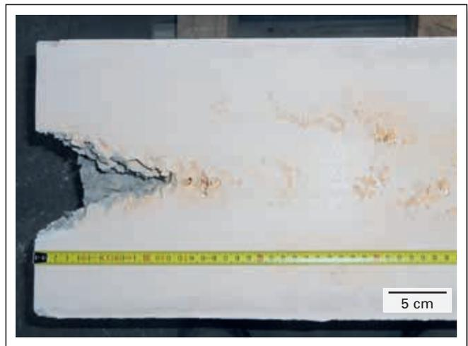
**Figure 8.** Longitudinal section of the cut CRB, with a clearly visible cavity followed by a porous region.
