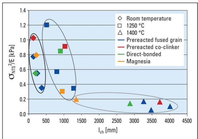
Figure 6. Relationship between  $\sigma_{NTS}^2/E$  and the characteristic length,  $l_{ch}$ , for all the brick types examined at room temperature, 1250 °C, and 1400 °C.
