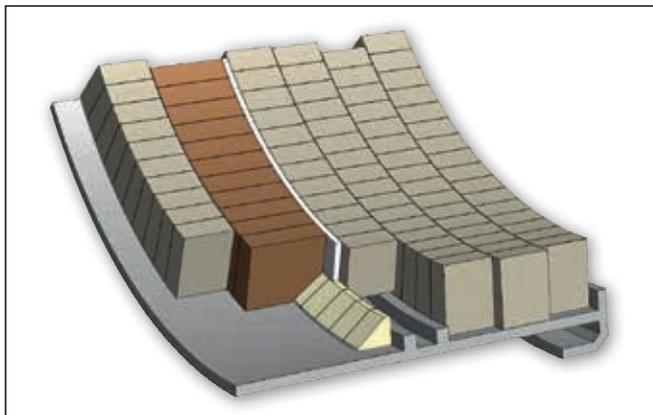
**Figure 1.** New RHI Thrust Lock System installed at a retaining ring, comprising special skew brick sets (cream and brown) and an expansion joint (white).
