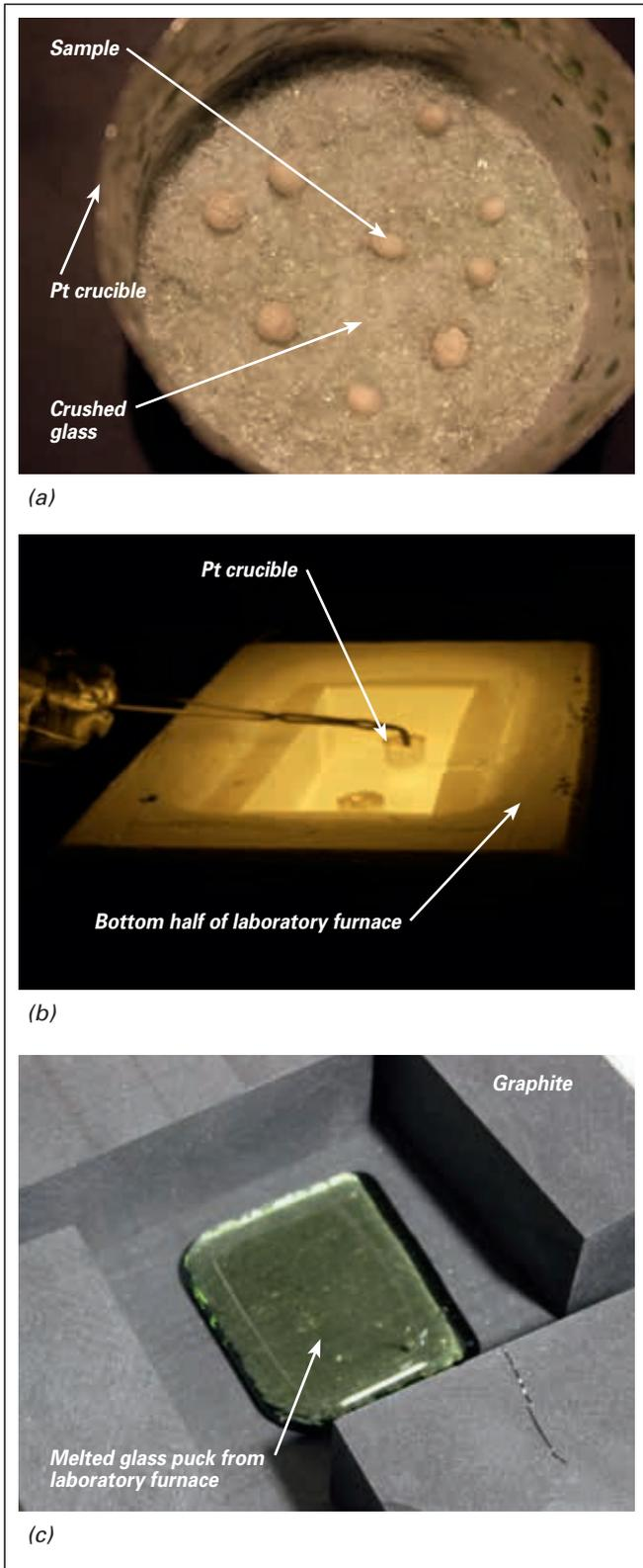
**Figure 9.** Laboratory furnace experiment with the chromite spinel colourant. (a) balls of sample colourant in soda-lime glass cullet within a platinum crucible, (b) platinum crucible placed in the laboratory furnace underneath the raised furnace lid, and (c) after the colourant was melted in the glass cullet it was poured into a graphite block mould to contain the glass as it cooled.
