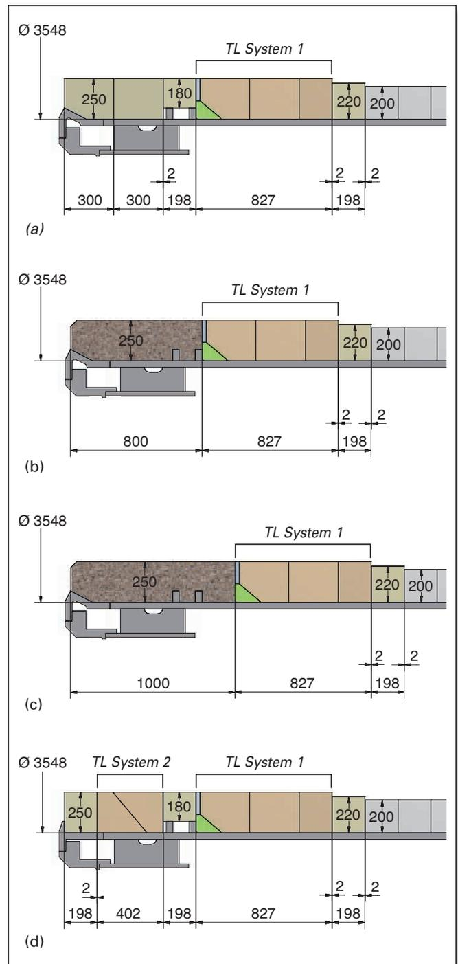
**Figure 3.** Different lining concepts: Thrust Lock (TL) System and (a) brick lining at the outlet, (b) monolithic outlet, (c) extended monolithic outlet, and (d) second TL System step. Dimensions are in mm.
