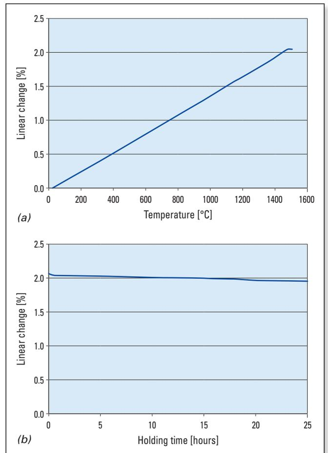
**Figure 4.** ANKER DG1. (a) linear change from room temperature up to 1500 °C and (b) creep in compression at 1500 °C over 25 hours.
