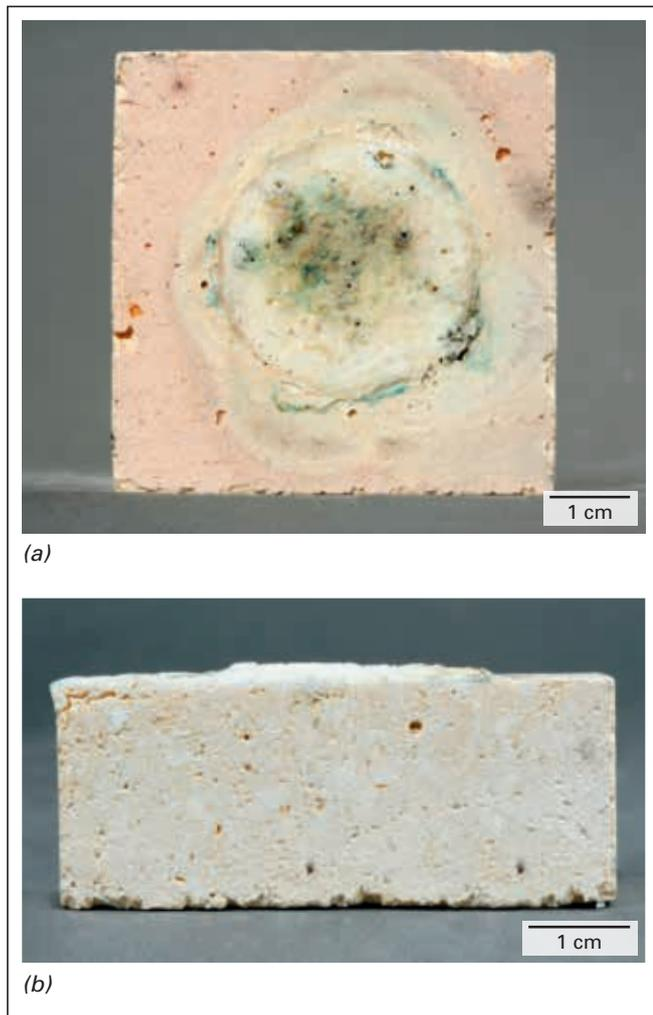
**Figure 4.** DIDURITAL AZ52 test sample after alkali attack. The test was performed in sodium carbonate vapour at 1370 °C for 72 hours. (a) surface and (b) cut sample.
