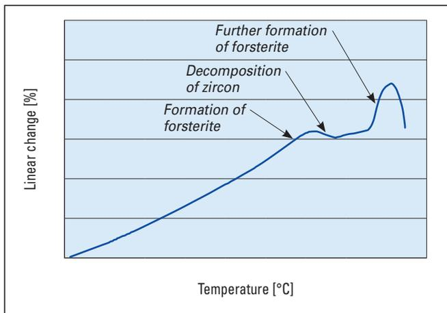
**Figure 6.** Firing behaviour of magnesia zircon.
