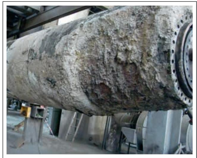
**Figure 4.** Burner lance after 5 months in operation demonstrating castable overheating at the burner tip. The burner tip was lined with a conventional low-cement castable. The adjacent segment was lined with a sol-bonded high-alumina castable and clearly shows less wear.
