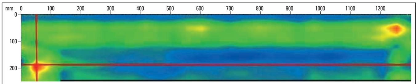
**Figure 10.** Ultrasound image of the CRB. The red coloured area (close to the intersecting red lines) indicates the presence of a cavity. The various other colourations are signal interferences and are not related to block flaws.
