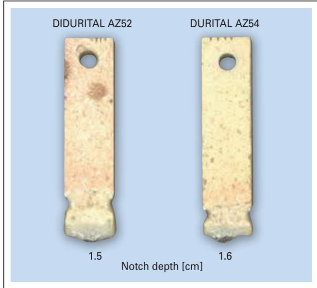
**Figure 3.** Static plate corrosion test comparing DIDURITAL AZ52 with the equivalent pressed DURITAL AZ54 grade for 96 hours at 1400 °C in soda-lime glass.
