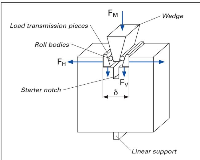
**Figure 2.** Principle of the wedge splitting test according to Tschegg under uniaxial loading [5].
