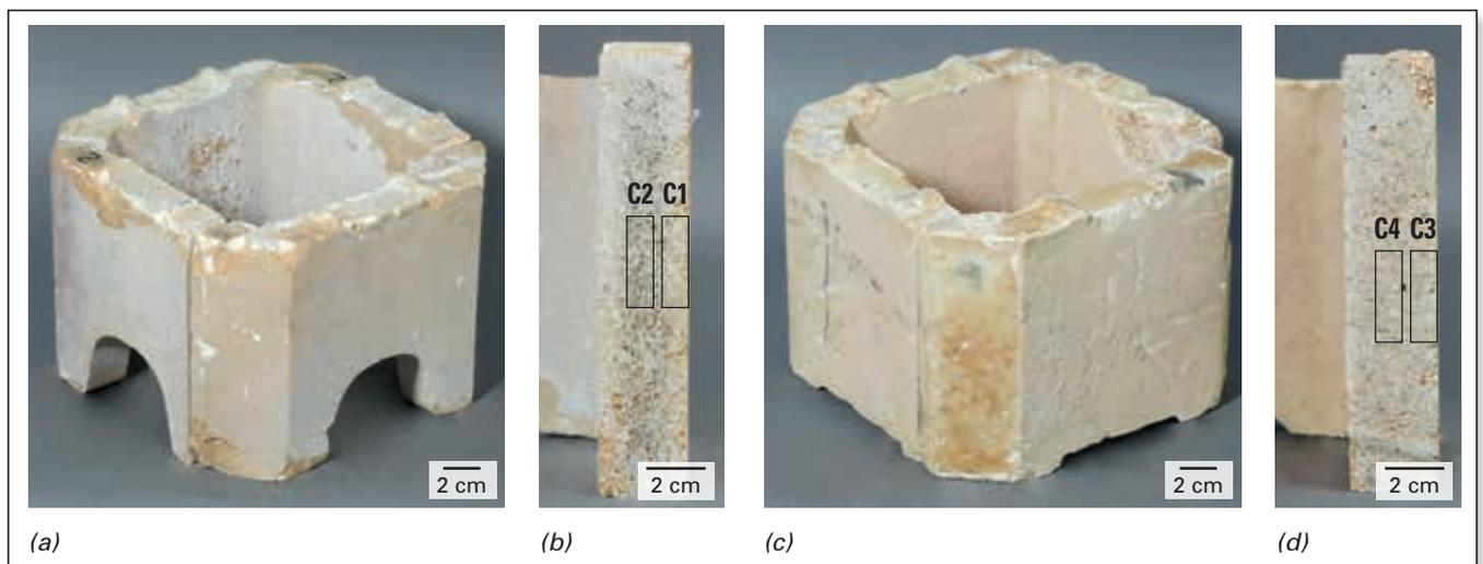
**Figure 9.** Postmortem samples for testing and analysis. (a,b) ANKER DG1 and (c,d) RUBINAL EZ. The analysis positions at the hot face and mid-brick region are indicated by the rectangles.
