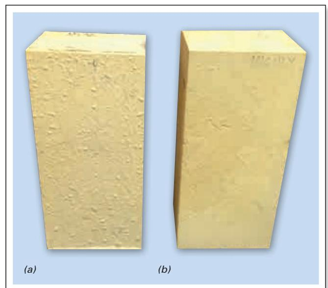
**Figure 2.** (a) standard 33 wt.% ZrO<sub>2</sub> AZS block after the door test at 1550 °C for 72 hours and (b) REFEL 1616ULX after the door test at 1550 °C for 72 hours followed by a further 5 cycles of 2 hours each. Glassy phase is clearly visible on the standard material while the REFEL 1616ULX block surface is absolutely dry. The sample dimensions are 300 mm x 150 mm x 100 mm.
