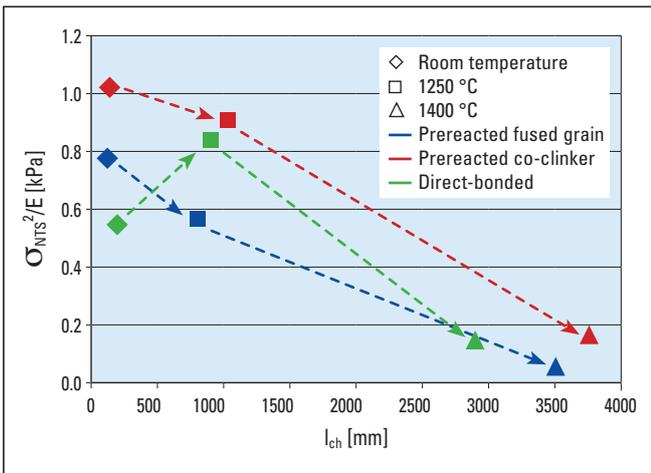
**Figure 7.** Comparison of the relationship between  $\sigma_{NTS}^2/E$  and the characteristic length,  $l_{ch}$ , for the MCr 50 types examined at room temperature, 1250 °C, and 1400 °C.
