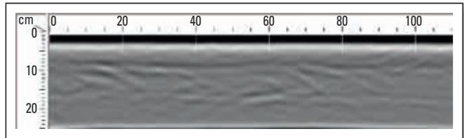
**Figure 6.** Radar image of the FVB. A smooth image without signal interferences indicates the absence of any cavity.
