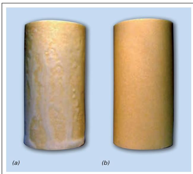
**Figure 1.** Samples after TC11 exudation testing (10 cycles). (a) standard 33 wt.% ZrO<sub>2</sub> AZS showing exudation (b) and almost zero exudation of REFEL 1616ULX. The sample dimensions are 50 mm in diameter x 100 mm high.
