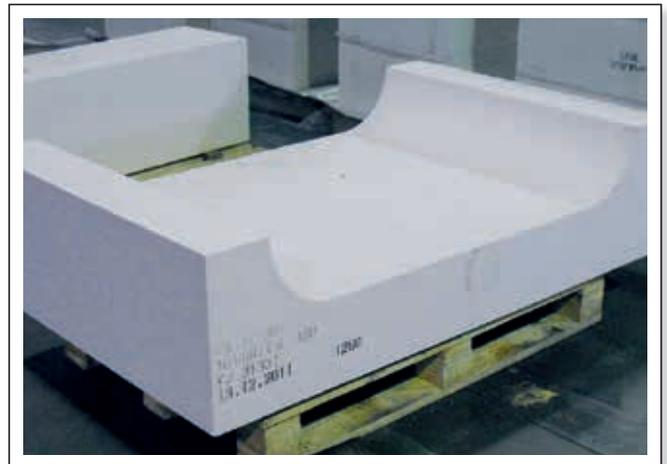
**Figure 5.** Feeder channel manufactured from DIDURITAL A98.
