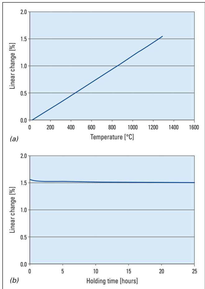
**Figure 7.** RUBINAL EZ. (a) linear change from room temperature up to 1300 °C and (b) creep in compression at 1300 °C over 25 hours.
