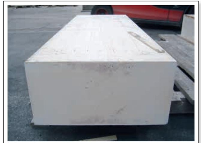
**Figure 4.** Cut face between the block and casting header of the FVB without any cavity. Cross section  $250 \times 500 \text{ mm}^2$ .
