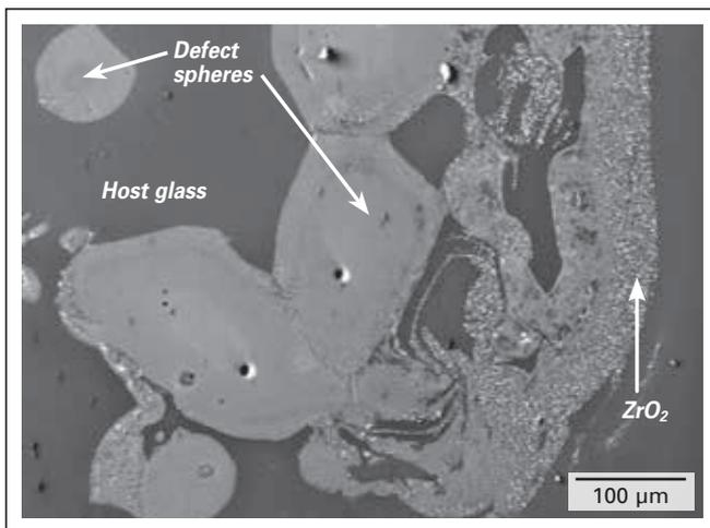
**Figure 2.** SEM backscattered electron image of the round defects and secondary zirconia from these round defects.
