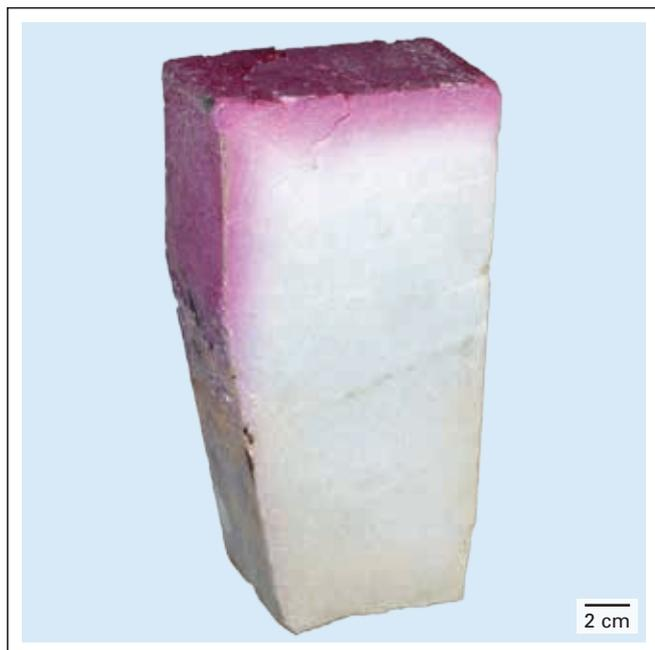
**Figure 6.** Sample of DURITAL K99EXTRA after 2 years in operation.
