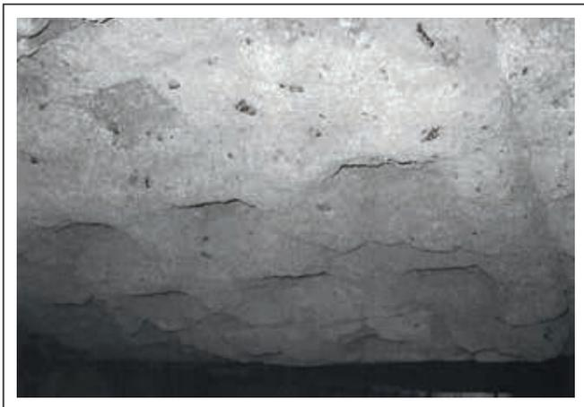
**Figure 2.** Bullnose with severe damage after 7 months in operation. Lining with a hydraulically bonded low cement high alumina gunning mix with additives of zirconium oxide and SiC.
