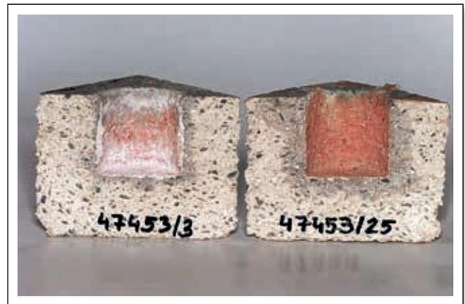
**Figure 8.** Cross section of crucible after 7 cycles of the crucible infiltration test, infiltration depth, RESISTAL B50ZIS (impregnated, left) and RESISTAL B50Z (not impregnated, right).
