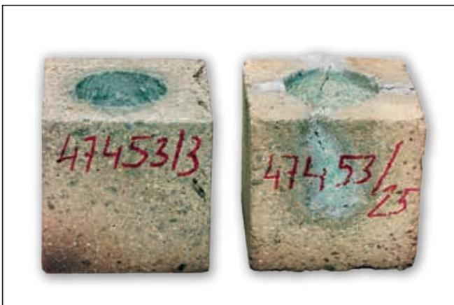
**Figure 7.** Crucible after 7 cycles of the crucible infiltration test, RESISTAL B50ZIS (impregnated, left) and RESISTAL B50Z (not impregnated, right).
