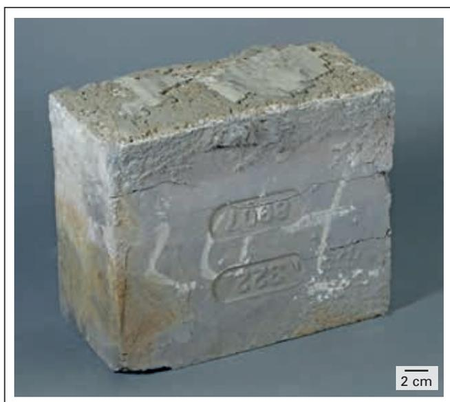
**Figure 1.** Brick sample received for post mortem analysis. The sample location was 7 meters from the kiln inlet.
