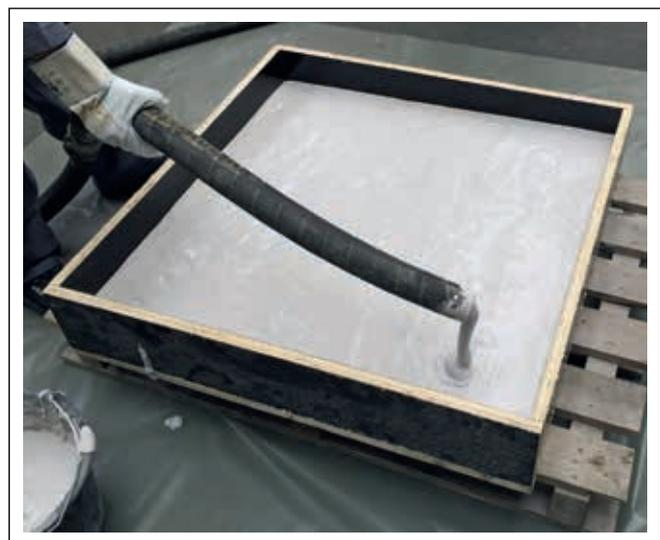
**Figure 2.** LEGRIT 143-1,2PC 0-1 pumped with 29% water into a flat mould. The consistency is very “creamy”. The mix can easily be densified by poking.
