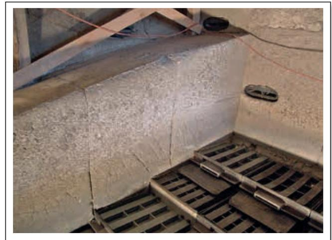
**Figure 6.** Clinker bed with CARSIT SOL S30-6 after 7 months in operation.
