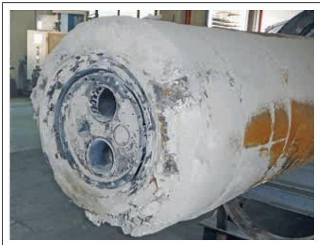
**Figure 8.** COMPAC SOL MB A100-15 after 7 months in operation.
