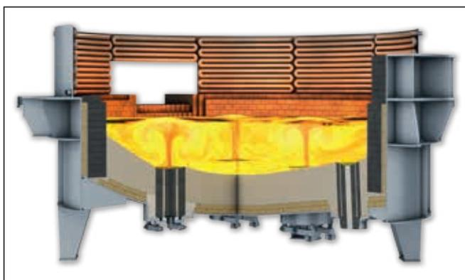
**Figure 1.** Efficient mixing throughout the steel melt using 3 gas purging plugs in the EAF hearth (Figure based on computational fluid dynamic (CFD) modelling of steel flow pattern).
