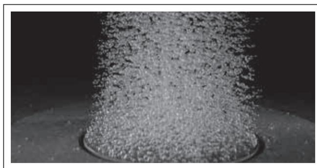
**Figure 2.** Bubble formation from a porous plug at a flow rate of 10 l/min.
