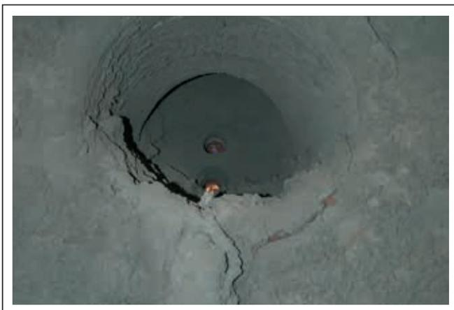
**Figure 5.** Build up of iron ore dust and melt within a combustion chamber.
