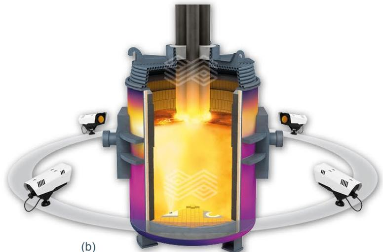
For the RH degasser in general, the most critical area besides the snorkel, is the conjunction between the bottom and wall up to the level of the alloying chute. The snorkels are immersed into the steel during the treatment and therefore not suited for online detection. Direct output of such a setup on the shop floor level is a monitoring and alarming system for immediate action.
