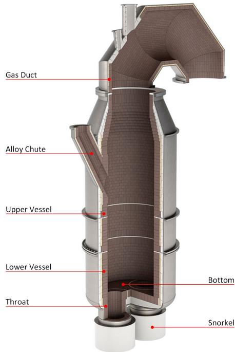
Figure 1: Schematic view of a RH degasser [16,18].
