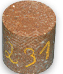
Magnesia brick with “HR” Technology after 600 hours in the steam chamber
