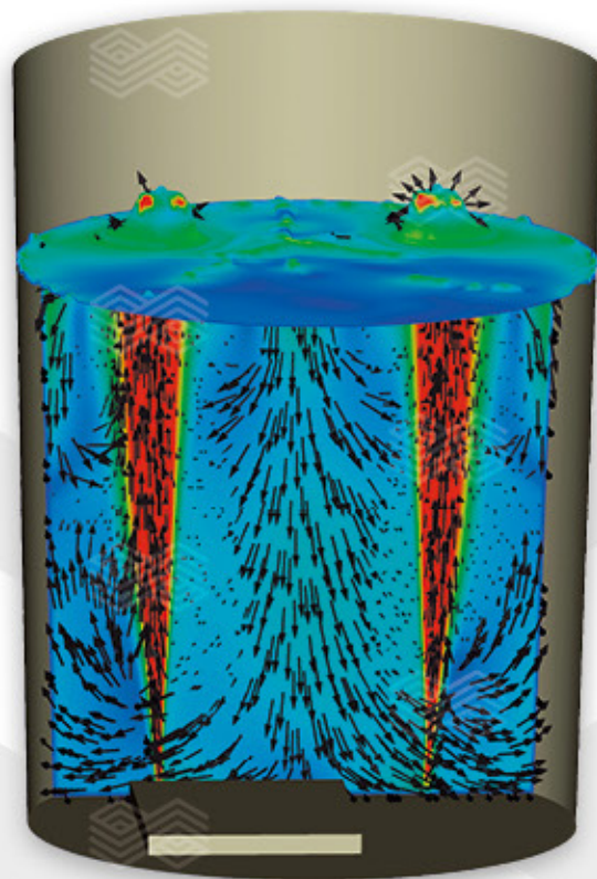
Ladle purging — flow patterns
