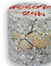
Magnesia brick not impregnated after 24 hours
