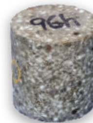
Magnesia brick with “R1” impregnation after 96 hours
