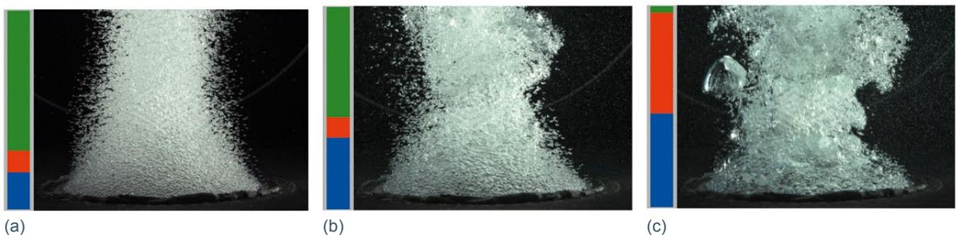
Photos taken with a high-speed camera showing the bubble formation at the plug surface of a large porous plug at 50 l/min, 250 l/min, and 500 l/min are given in Figure 7. A visual, qualitative comparison confirms a shift to larger bubble sizes with increasing flow rates. This is in good agreement with the vibration measurements of the bubble index, given to the left of each picture.
