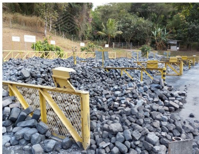
Figure 3. Carbide stabilisation using the weathering method.
