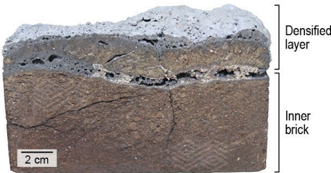
Figure 1. Cross-section of a magnesia-chromite brick after application showing severe slag infiltration and metallic phases at the hot face (densified layer) and the inner brick.
