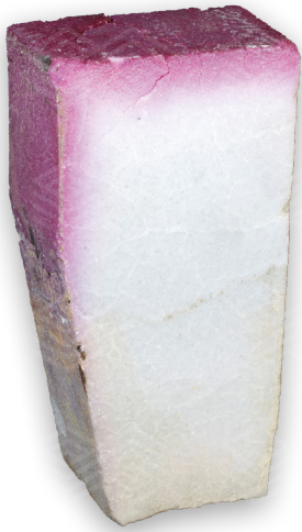
DURITAL CZ25P Sample after two years field test
