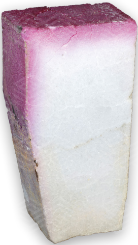
DURITAL C99 Sample after two years field test
